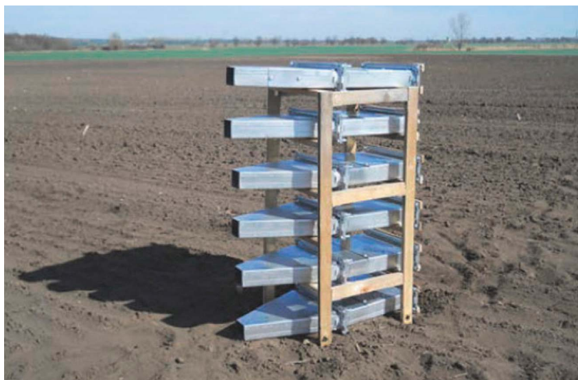
Figure 4 2 nd model of soil particle catcher Source: Urban, 2011
