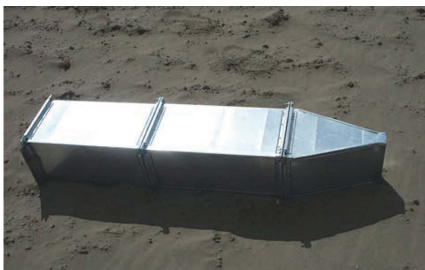
Figure 3 1 st model of soil particle catcher Source: Urban, 2011
